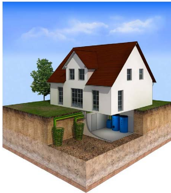
Figure 6: short vertical loops (from http://www.enbw.com [6])
