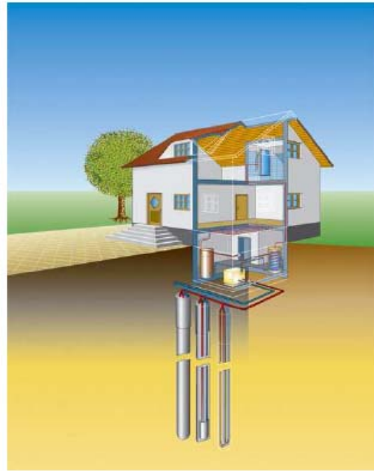
Fig. 1: Schematic sketch of vertical and horizontal oriented heat pipe installations (source)
