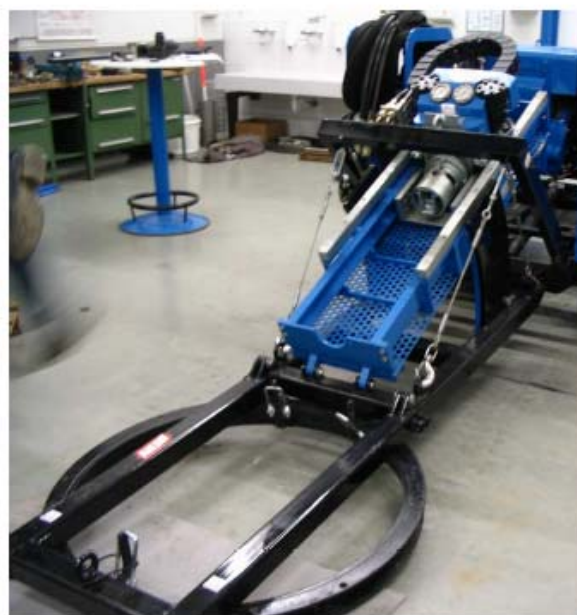
Fig. 5: The Geodrill 4 T with open rotary ring (left) and at a field testing operation (right; drill performance 2-4 min /metre in shale and paleozoic sandstone)
