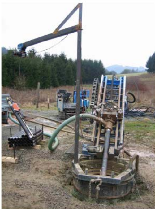
Fig. 5: The Geodrill 4 T with open rotary ring (left) and at a field testing operation (right; drill performance 2-4 min /metre in shale and paleozoic sandstone)
