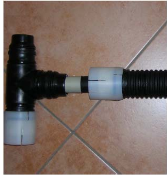
Fig. 6: State-of-the-art coaxial ground source heat exchangers that are easy to connect due to a click-system. The cold brine coming from the heat pump flows through the inner pipe down to the bottom of the heat exchanger and ascends at the inner side of the outer pipe back to the heat pump.
