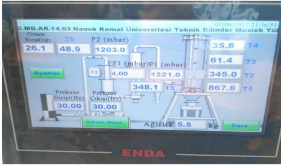
Figure 6. Measurement and control equipment display screen
