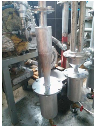
Figure 3. Gas cleaning system (Aktaş et al., 2017)
